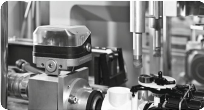
Monitoring the negative pressure ensures the correct positioning of the components during fully automatic assembly of gas meters.
