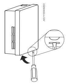
2. Take off the module by hand and replace it with a new one.
