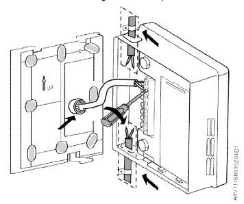
**4.** Attach the housing to the mounting plate at the top and then snap on the housing at the bottom.
