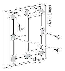
**3.** Connect and screw wires correctly to the terminal. For surface mounting, you must break out the wiring hole at the top or bottom first.
